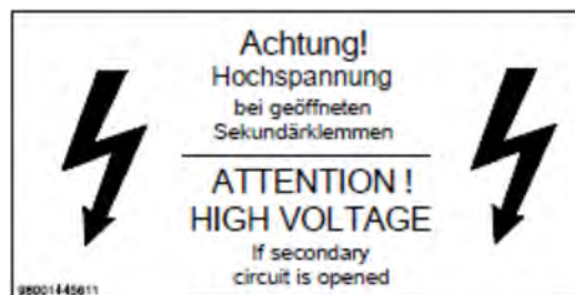
Fig. 30: Never operate the secondary terminals without burden.
