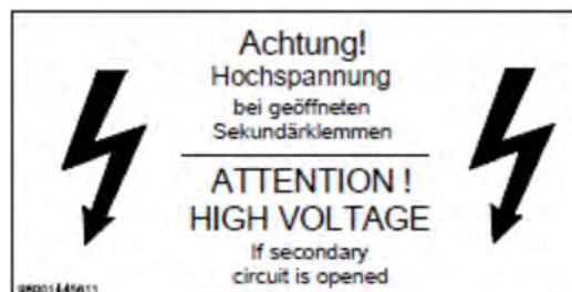
Fig. 28: Never operate the secondary terminals without burden!
