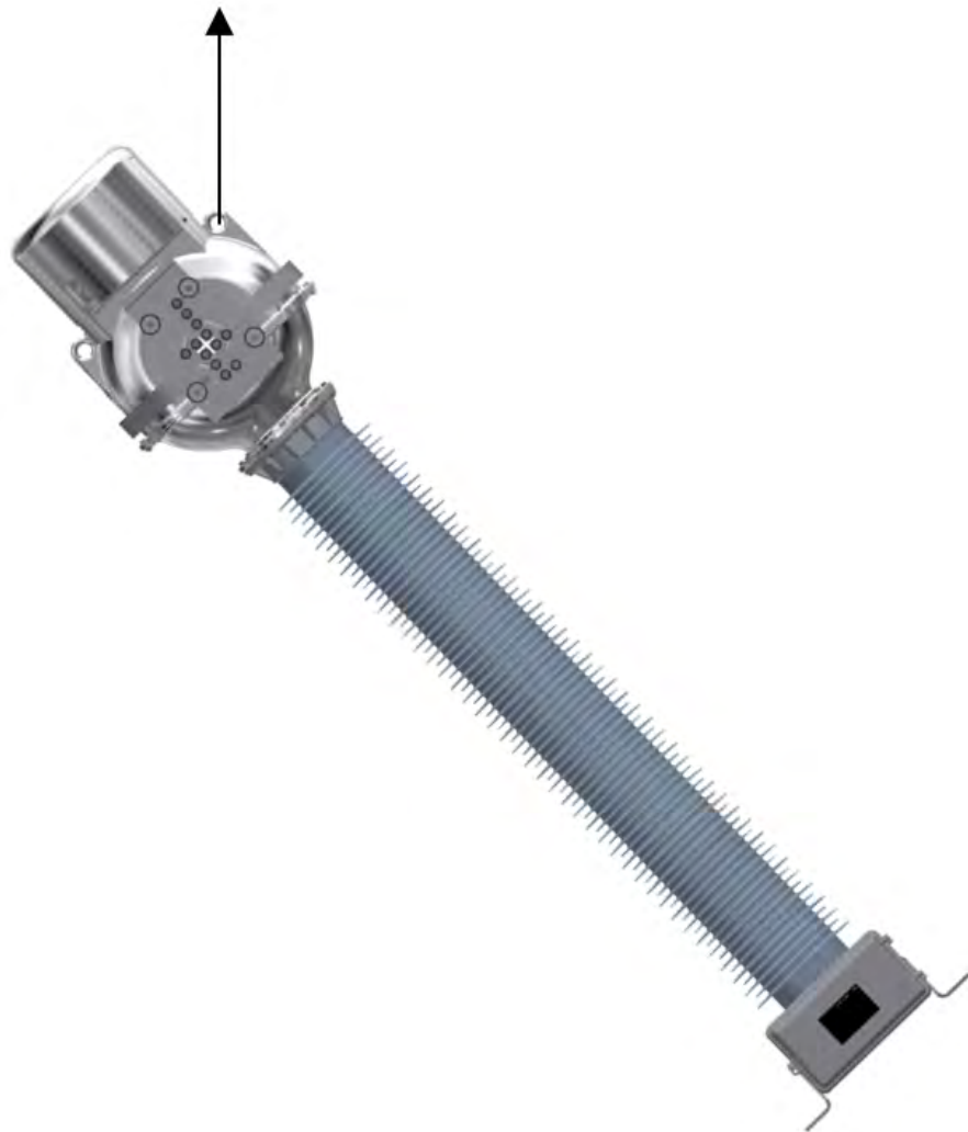
Fig. 21: Standing the ICO type current transformer up
