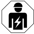
Fig. 2: Working with the device only permitted for electrotechnical qualified personnel
